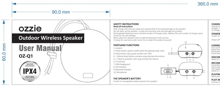
Connect the supplied charging cable to the charge input and to a USB port on your computer or a USB charger. The charging LED is lift red during charging. The LED turns off when fully charged.It is recommende to charge 10 minutes befroe power on if you days.
