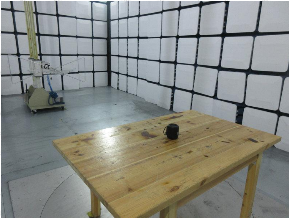
Photo of Radiation Emission Test
