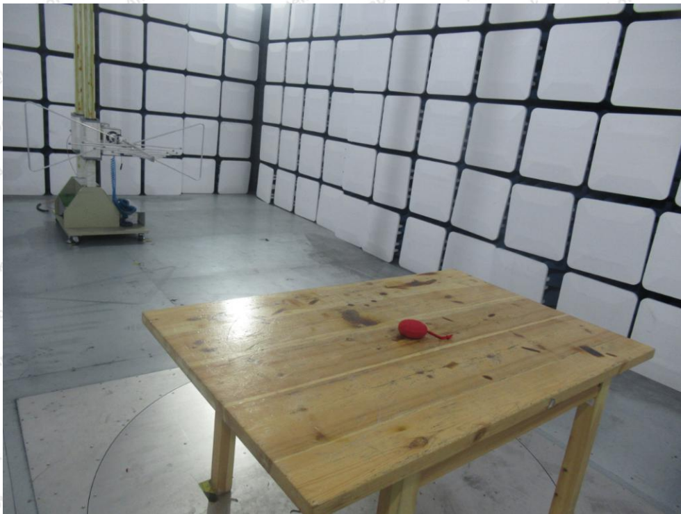
Photo of Radiation Emission Test
