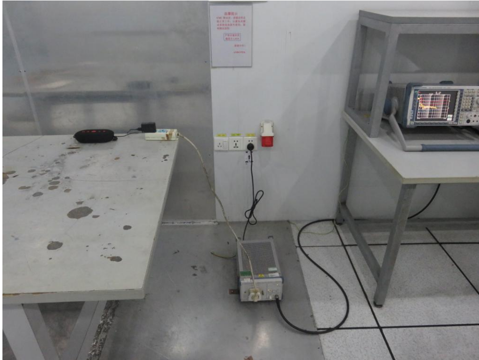
Photo of Conducted Emission Measurement
