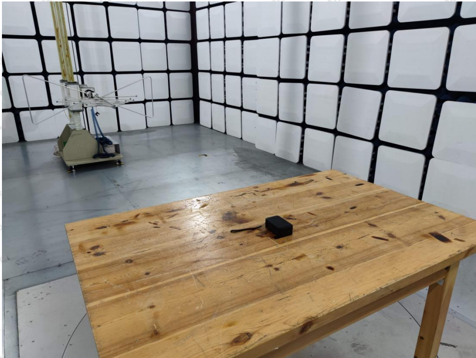
Photo of Radiation Emission Test
