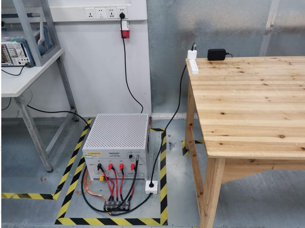
Photo of Conducted Emission Measurement
