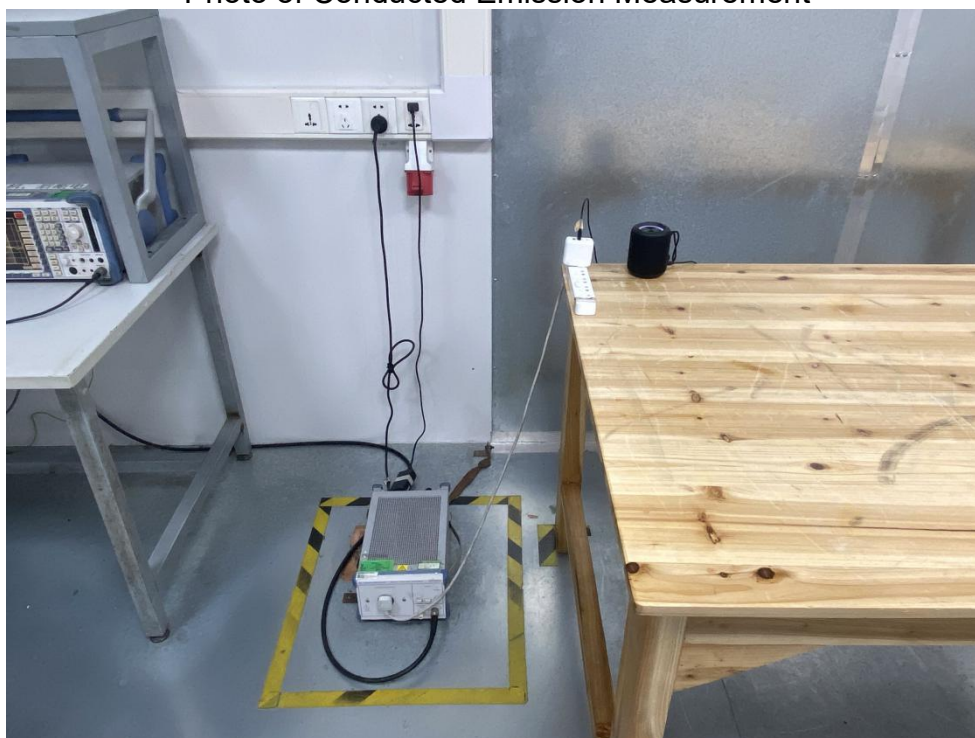
FCC ID: 2AL7B-OZ-E100MINI Photo of Conducted Emission Measurement
