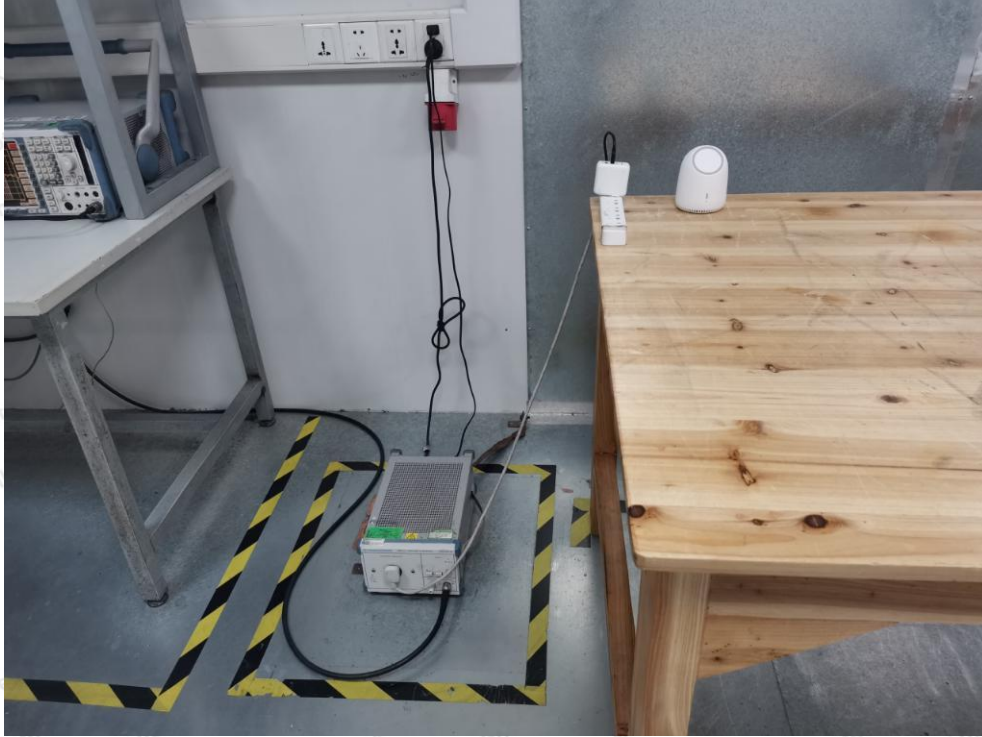
Photo of Conducted Emission Measurement
