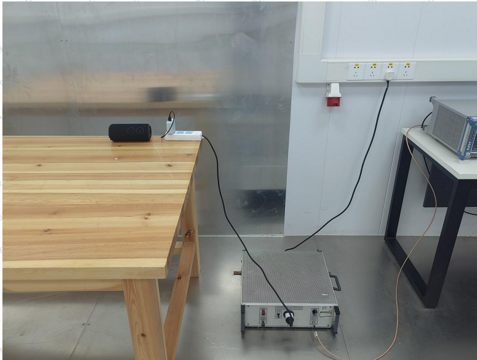
Photo of Conducted Emission Measurement
