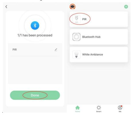
If you haven't seen the newly added device in the main interface, you can pull down to refresh. When there are multiple devices, you can add them one by one as described above, or select Auto Search to add device. You can refer to the instruction manual of Yankon Smart Lighting for details.
