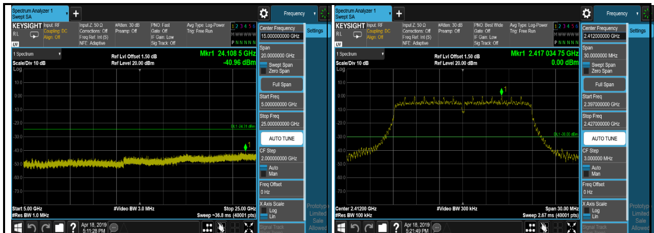
802.11n(HT20),2412MHz,Ant1,Plot 2,Band Edge
