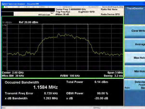
20dB Bandwidth plot on channel 78 (3Mbps)
