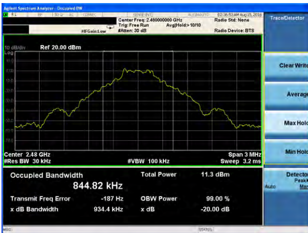
20dB Bandwidth plot on channel 78 (1Mbps)
