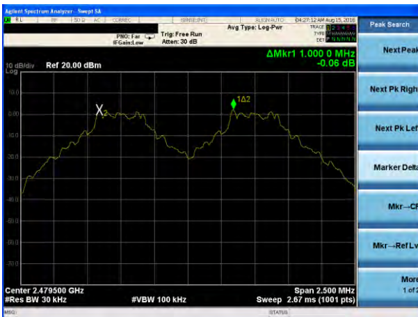
(1Mbps) Channel Separation plot on channel 77-78
