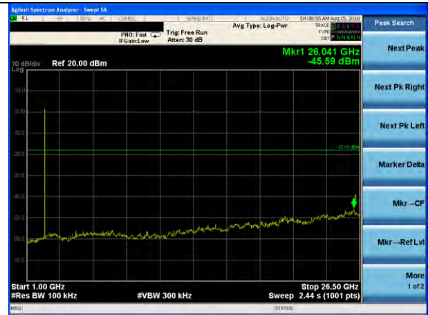
GFSK on channel 00
