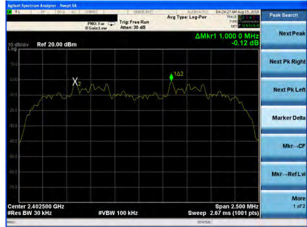
(2Mbps) Channel Separation plot on channel 39-40
