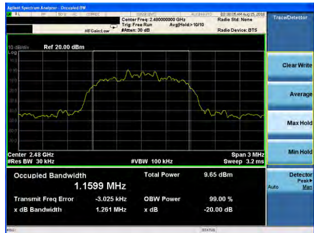
20dB Bandwidth plot on channel 78 (2Mbps)
