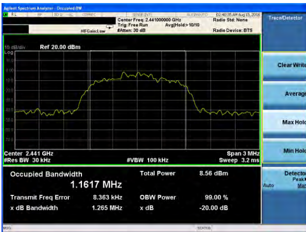
20dB Bandwidth plot on channel 39 (3Mbps)
