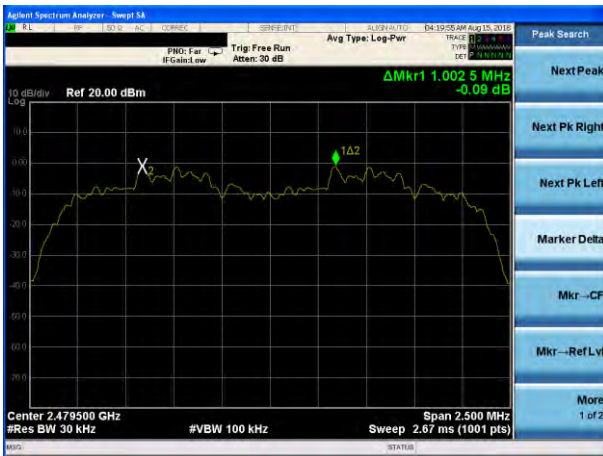
(3Mbps) Channel Separation plot on channel 77-78
