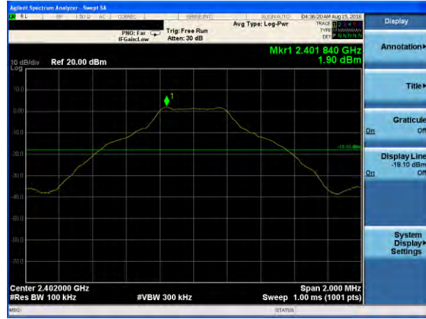
GFSK on channel 00
