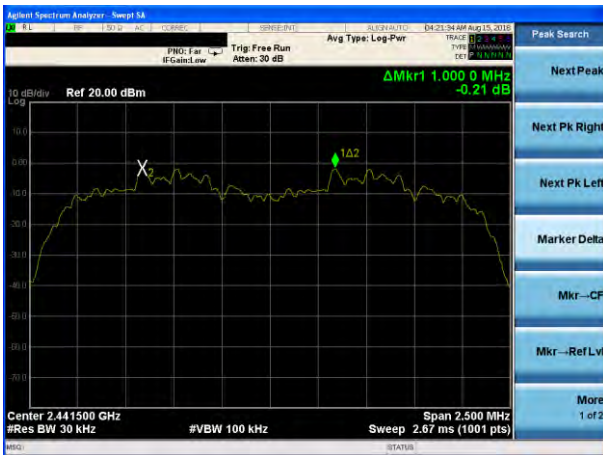
(3Mbps) Channel Separation plot on channel 39-40
