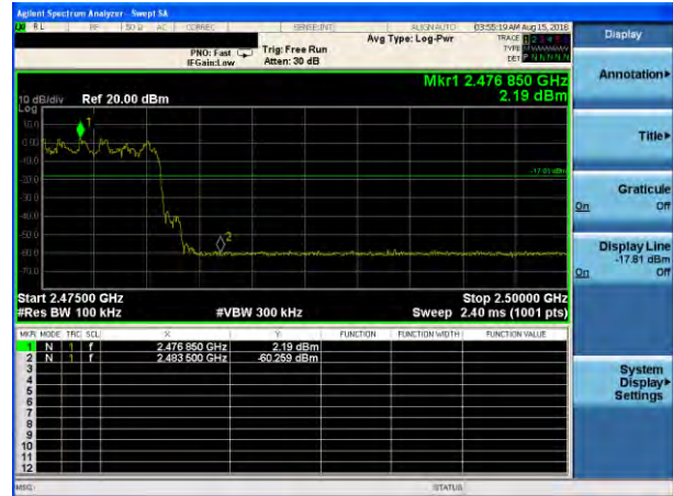
\pi /4-DQPSK: Band Edge-High Channel (Hopping Mode)
