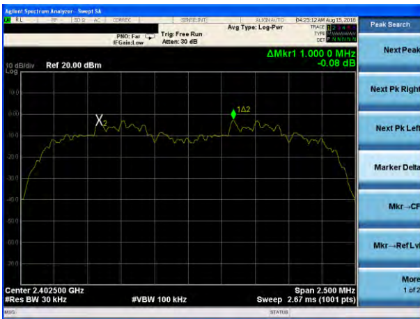
(3Mbps) Channel Separation plot on channel 00-01
