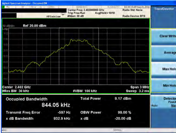
20dB Bandwidth plot on channel 39 (1Mbps)
