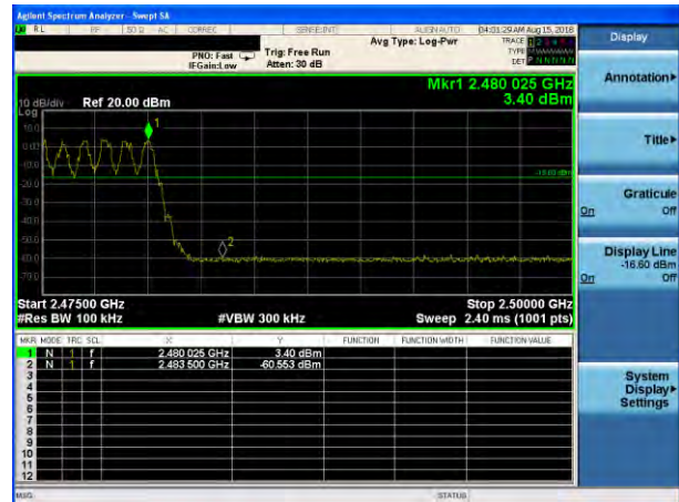
GFSK: Band Edge-High Channel (Hopping Mode)
