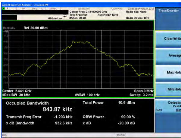
20dB Bandwidth plot on channel 78 (1Mbps)
