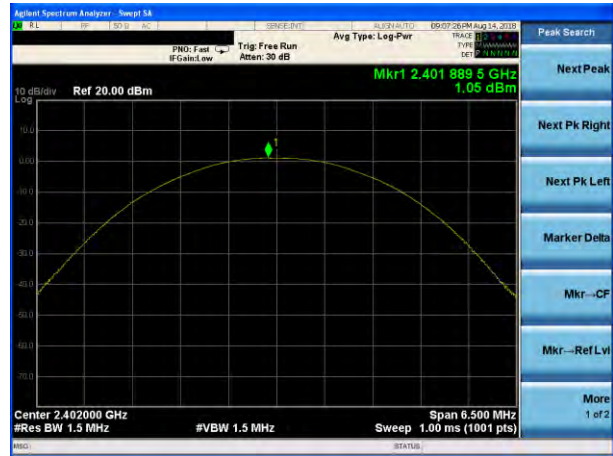
Peak output Power plot on channel 39 (2Mbps)
