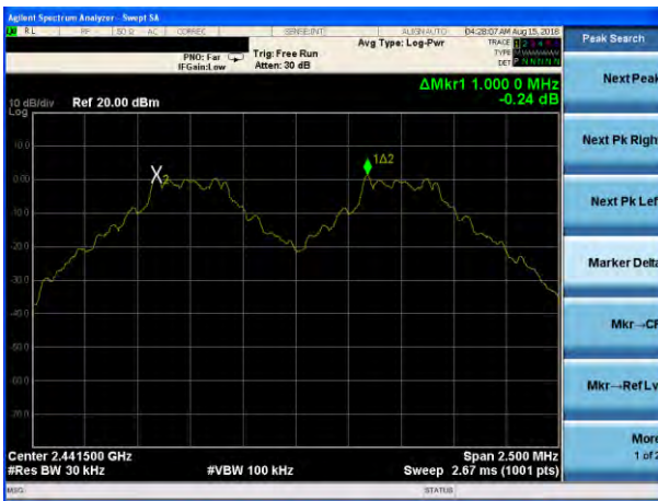
(1Mbps) Channel Separation plot on channel 77-78
