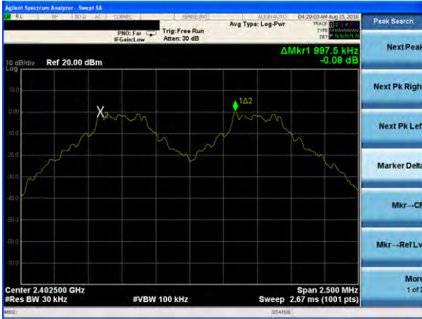
(1Mbps) Channel Separation plot on channel 39-40
