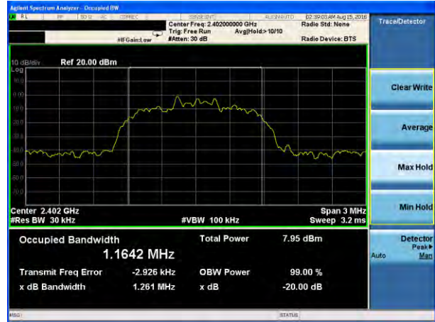
20dB Bandwidth plot on channel 39 (2Mbps)
