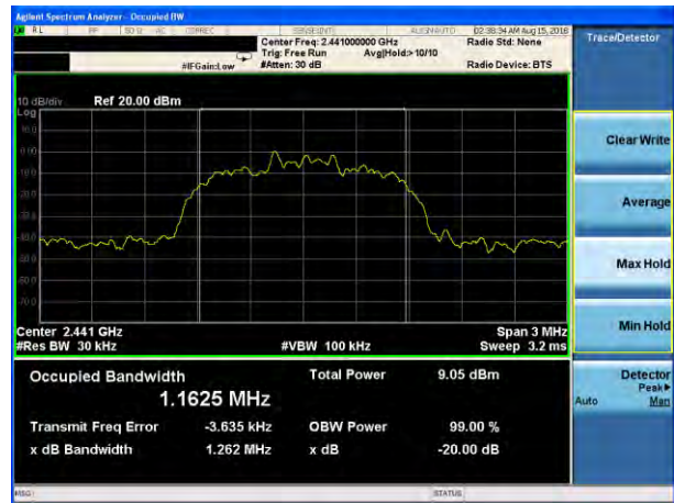
20dB Bandwidth plot on channel 78 (2Mbps)
