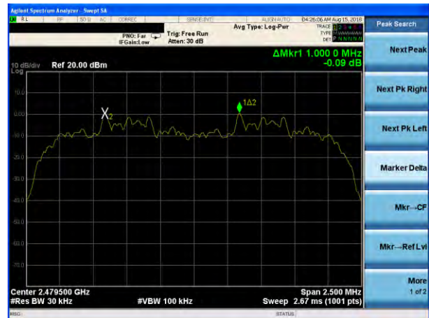
(2Mbps) Channel Separation plot on channel 77-78
