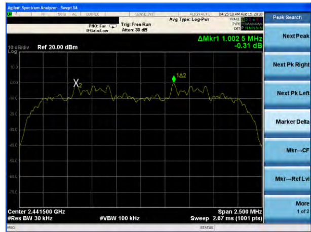
(2Mbps) Channel Separation plot on channel 77-78
