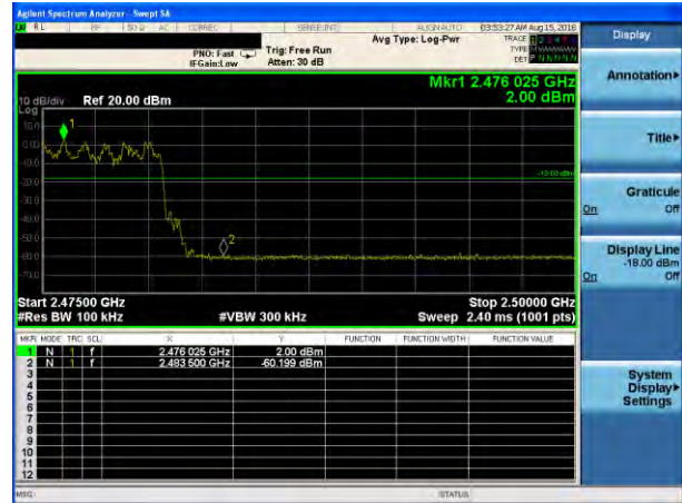
8-DPSK: Band Edge-High Channel (Hopping Mode)
