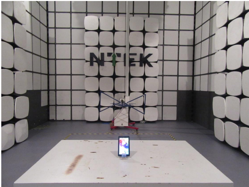
Radiated Measurement Photos(30MHz~1GHz )
