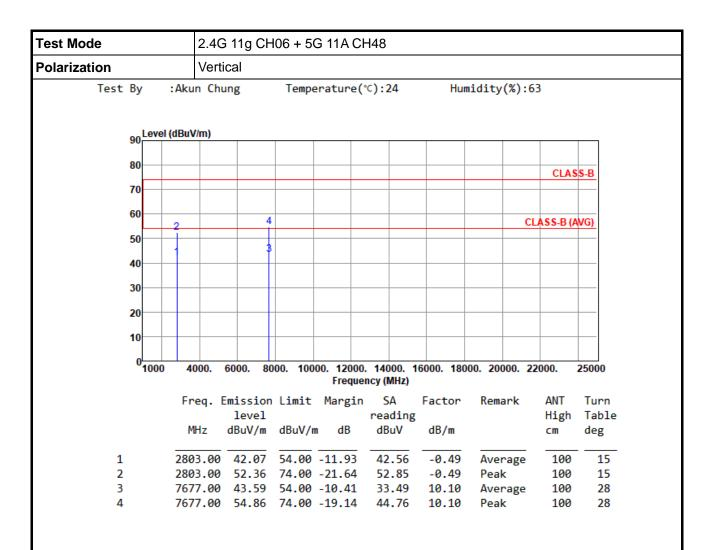
Note 1: Emission Level (dBuV/m) = SA Reading (dBuV) + Factor\* (dB/m)
