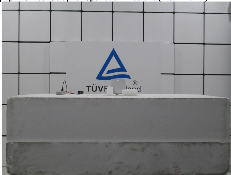
Photograph 10: Test Setup for Spurious Emissions (Front View 2)
