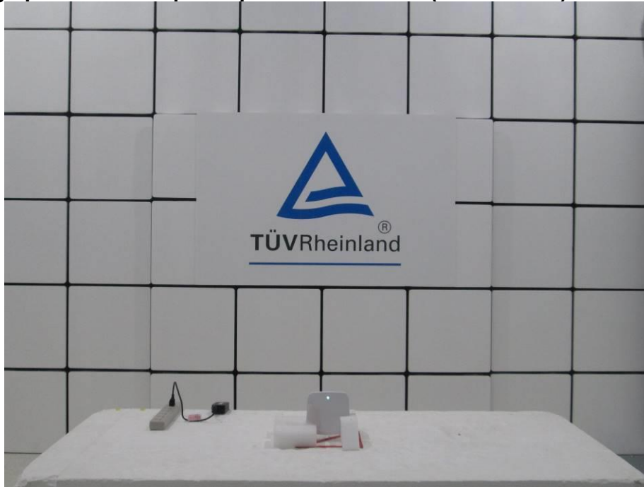
Photograph 10: Test Setup for Spurious Emissions (Front View 2)
