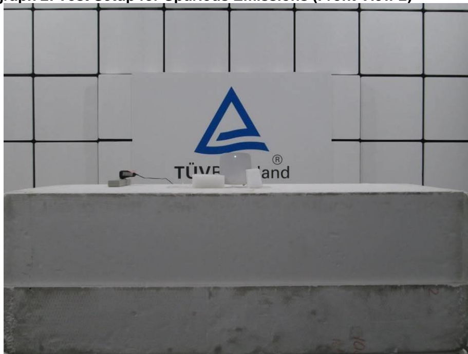
Photograph 2: Test Setup for Spurious Emissions (Front View 2)
