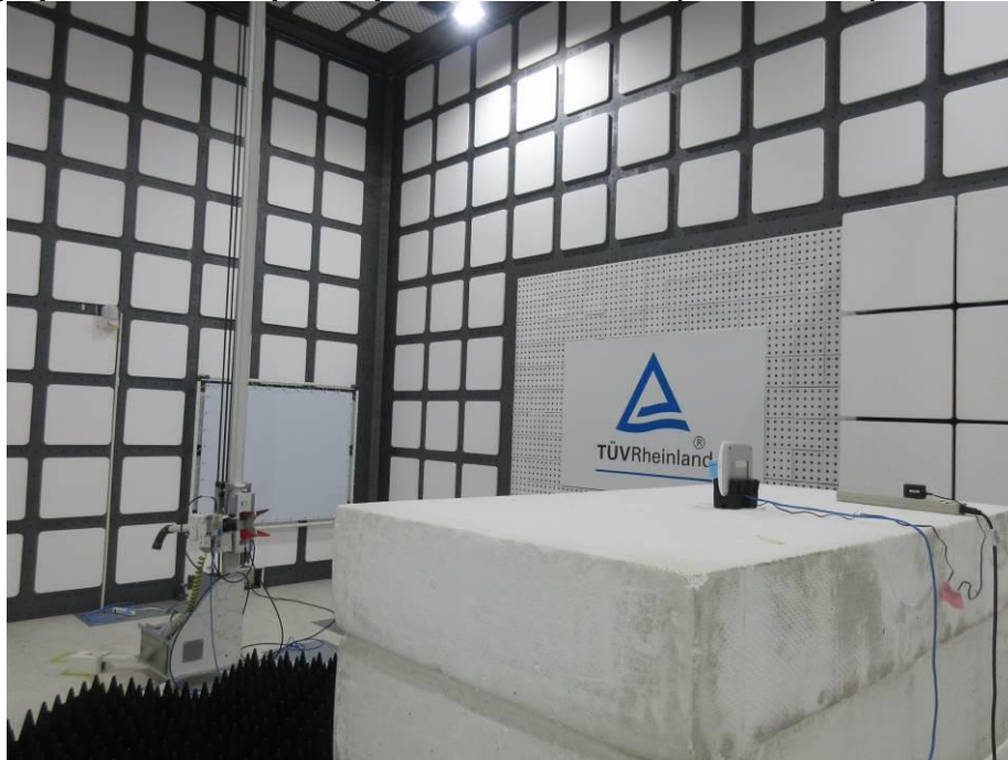
Photograph 6: Test Setup for Spurious Emissions (Back View 4)
