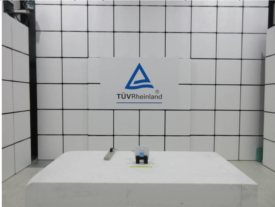
Photograph 2: Test Setup for Spurious Emissions (Front View 2)
