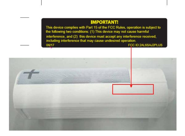
The rating label was sticked at the enclosure bottom of apparatus
