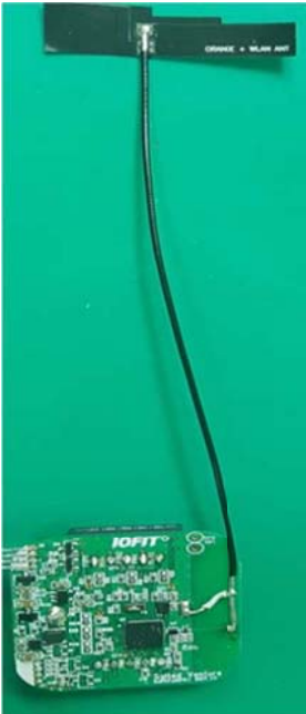
View of Antenna
