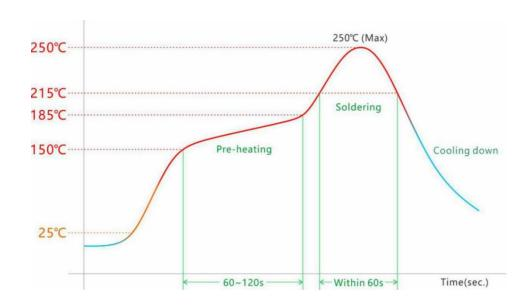
Please use the reflow within 2 times. Set up the highest temperature within 250℃.
