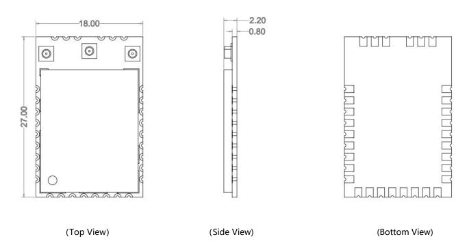
Module dimension: 27mm\*18mm\*2.2mm (L\*W\*H; Tolerance: ±0.15mm) IPEX / MHF-1 connector dimension: 3.0\*2.6\*1.2mm (L\*W\*H, Ø2.0mm)
