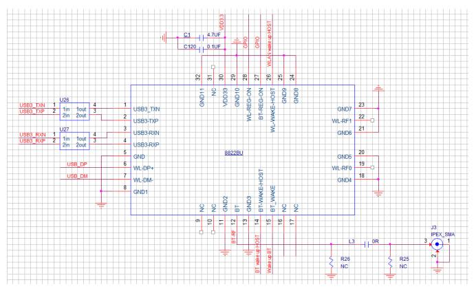
Figure 5-Typical application circuit
