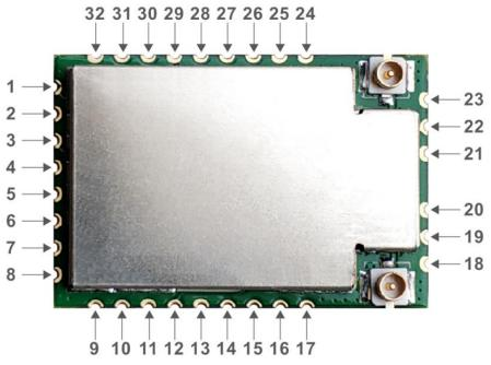
Figure 4-Pin Assignments (Top view)
