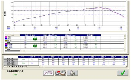
Figure 8 Typical Solder Reflow Profile
