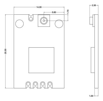
Module dimension: 20.3\*14.0\*2.35mm(L\*W\*H; Tolerance: ±0.15mm)
