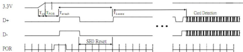
Figure 4. RTL8723DU USB Bus Power On Sequence
