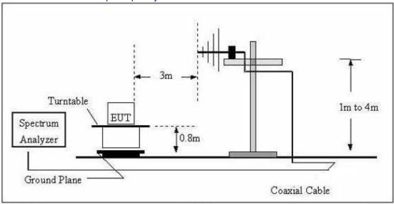
(C) Radiated Emission Test-Up Frequency Above 1GHz
