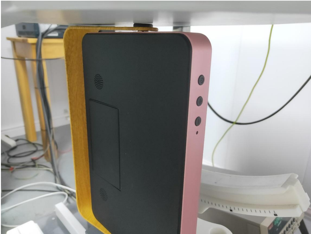
0mm body-worn Bottom Side Setup Photo
