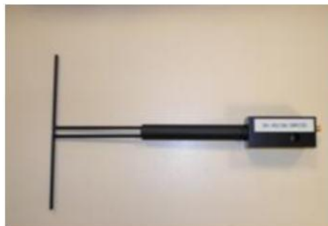
Figure 1 – Satimo COMOSAR Validation Dipole
