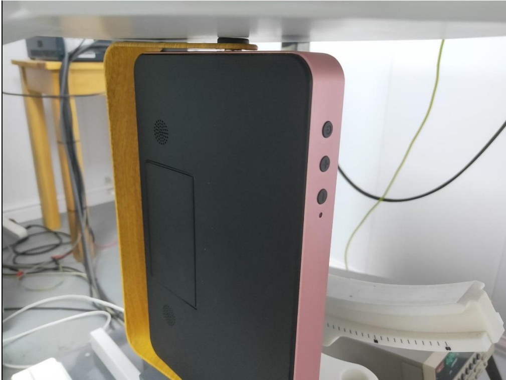
0mm body-worn Bottom Side Setup Photo
