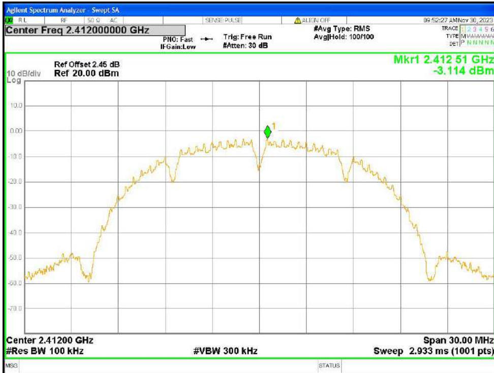
Tx. Spurious NVNT b 2412MHz Ant1 Ref
