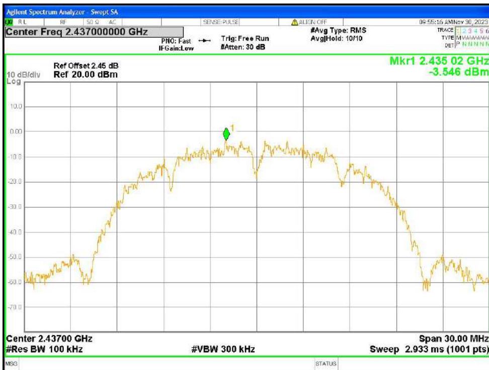
Tx. Spurious NVNT b 2437MHz Ant1 Ref
