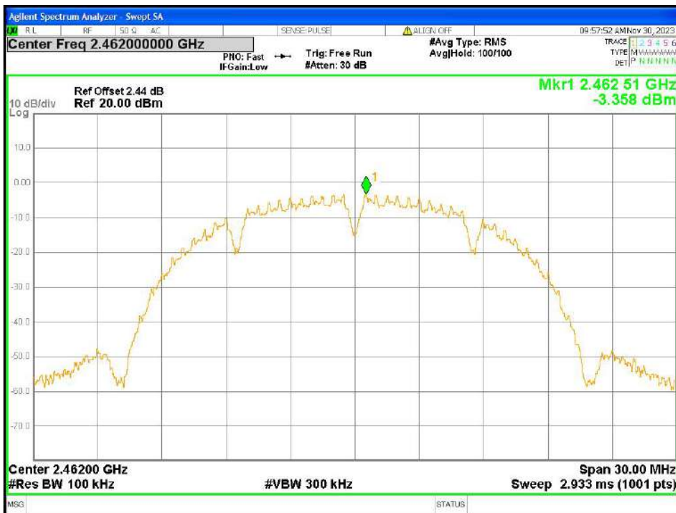
Tx. Spurious NVNT b 2462MHz Ant1 Ref
