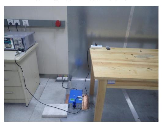
FCC RADIATED EMISSION TEST SETUP
