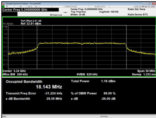
(802.11 ac20) 26dB Bandwidth plot on channel 48
