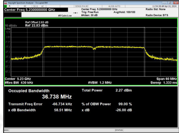
(802.11 n40) 26dB Bandwidth plot on channel 46
