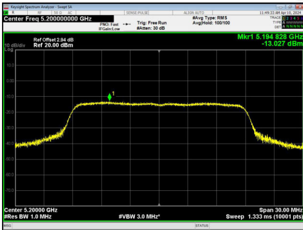
(802.11ac20) PSD plot on channel 40
