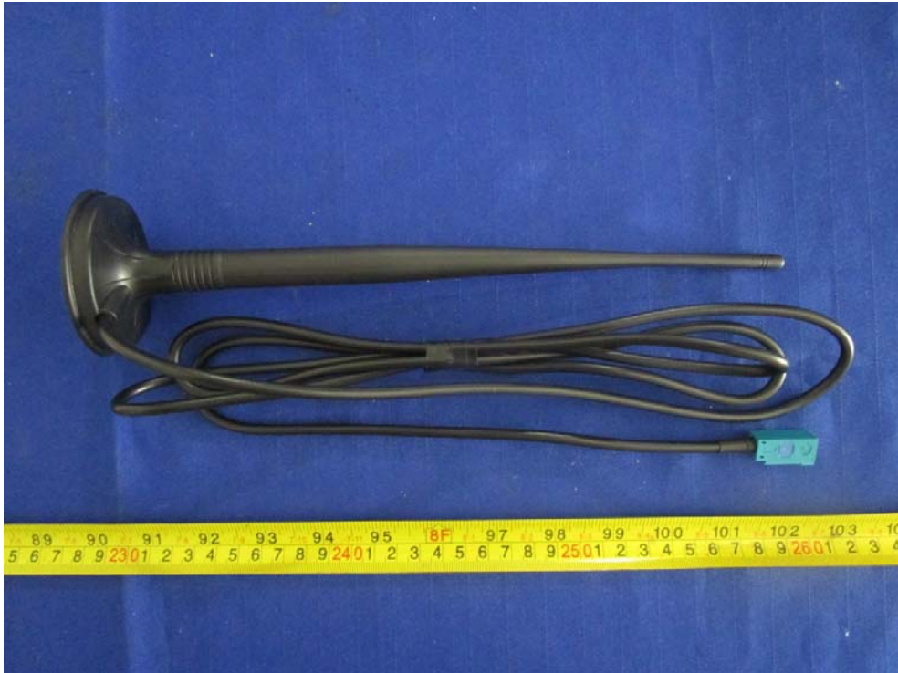
EUT – DSRC Antenna View
