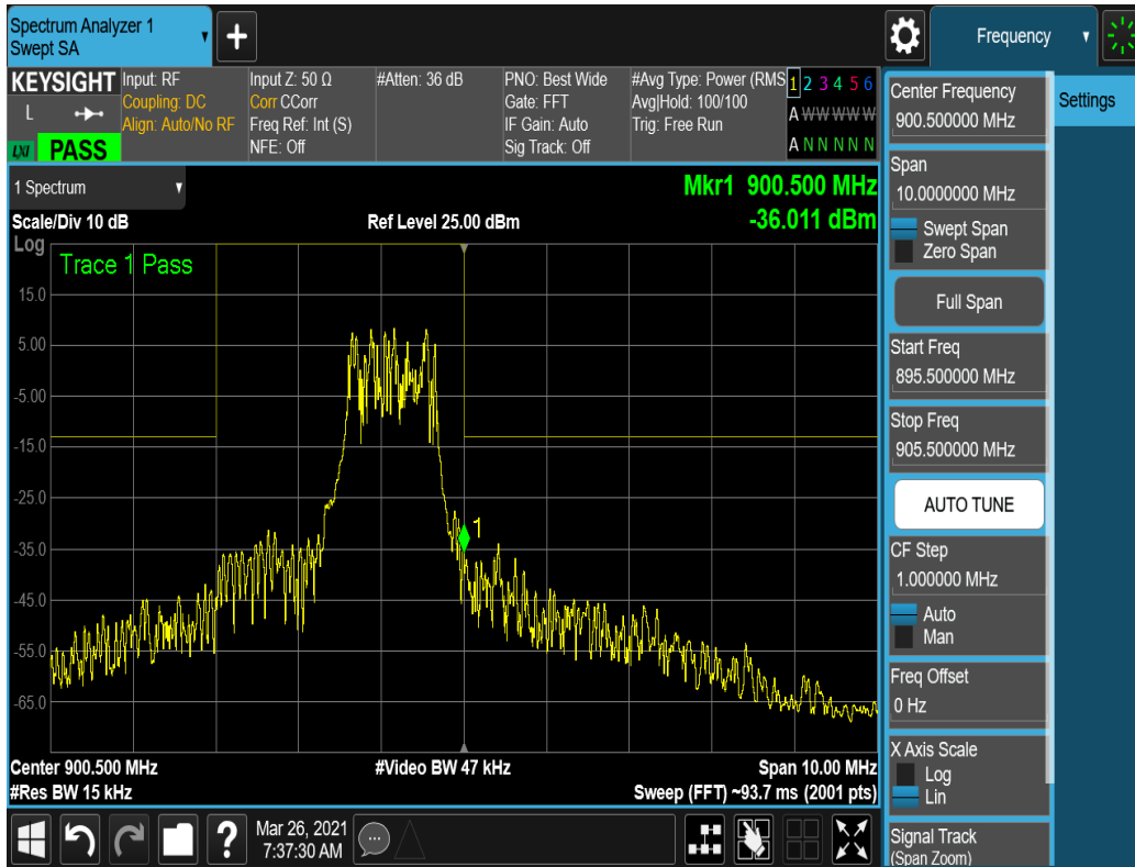
Plot 7-8. Upper Band Edge Plot (3MHz, QPSK, 6RB, RB Offset 0, NB=1)
