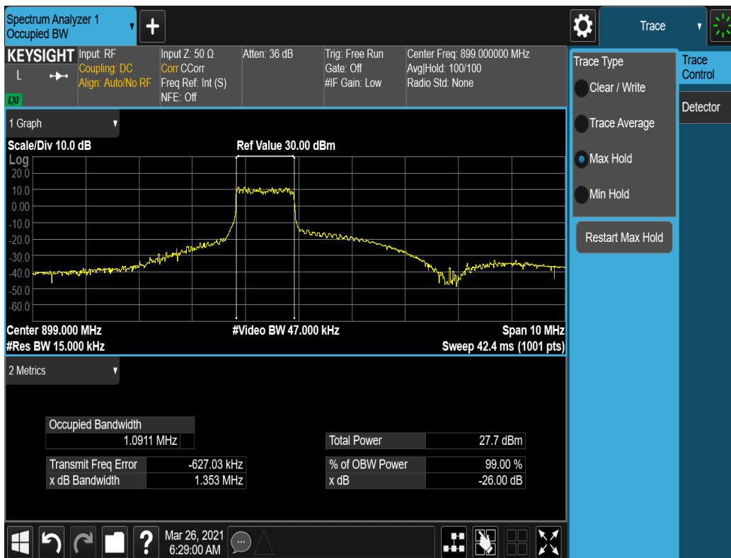
Plot 7-3. Occupied Bandwidth Plot (3MHz, 16QAM, RB 6, RB Offset 0, NB=0)
