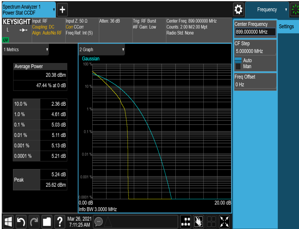
Plot 7-19. Peak to Average Ratio (3MHz, QPSK, RB 6, RB Offset 0, NB=0)
