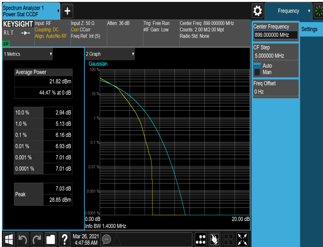
Plot 7-16. Peak to Average Ratio (1.4 MHz, 16QAM, 6 RB, 0 Offset)
