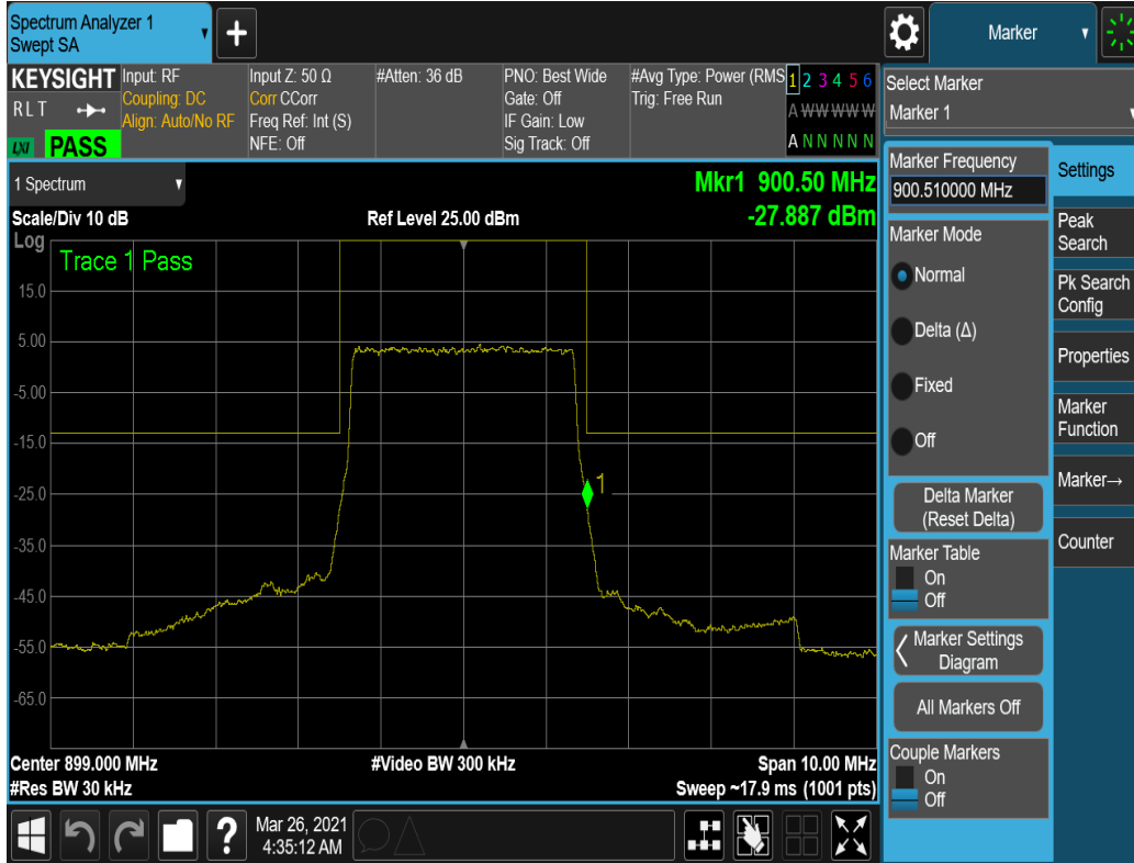
Plot 7-6. Upper Band Edge Plot (3 MHz, QPSK, 15 RB, 0 Offset)
