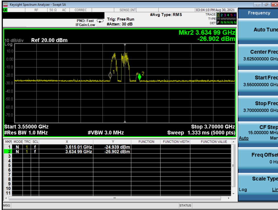
Plot 19. Conducted Measurement - UUT RF transmission range and bandwidths are less or equal to frequency range and bandwidth of compatible BTS-CBSD (WINNF.FT.C.DRG.1)
