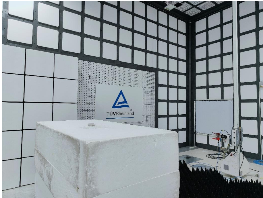
Photograph 6: Test Setup for Spurious Emissions (Back View 4)
