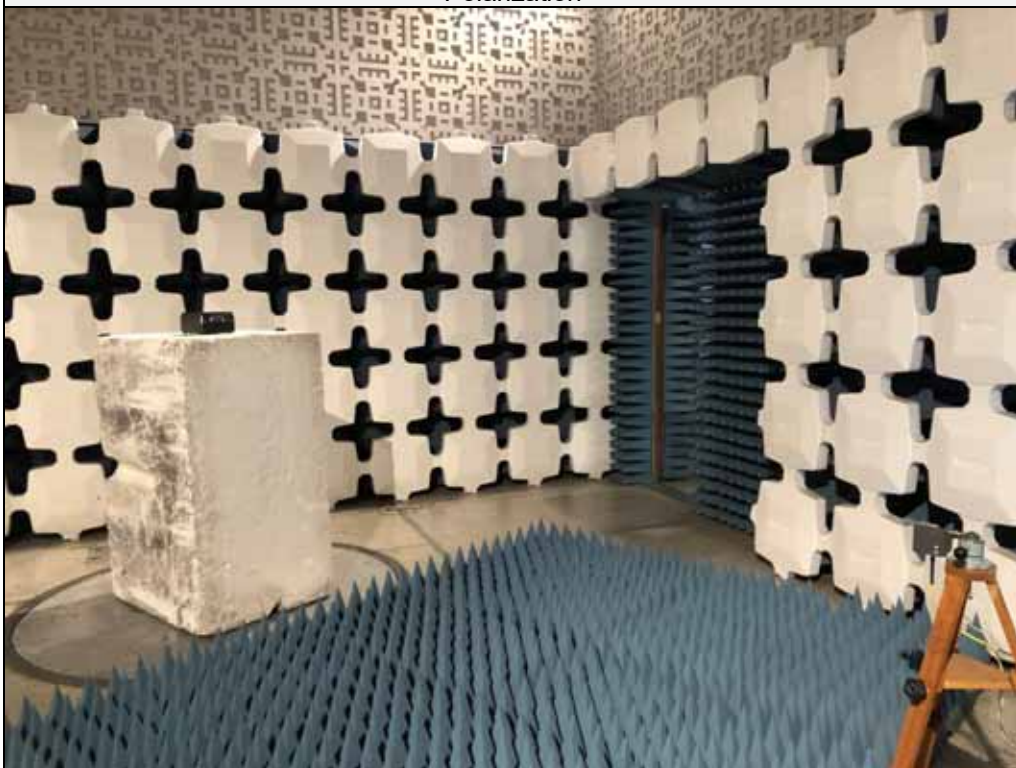
Test Setup for Radiated Spurious Emissions – 18-26.5GHz Vertical Antenna Polarization
