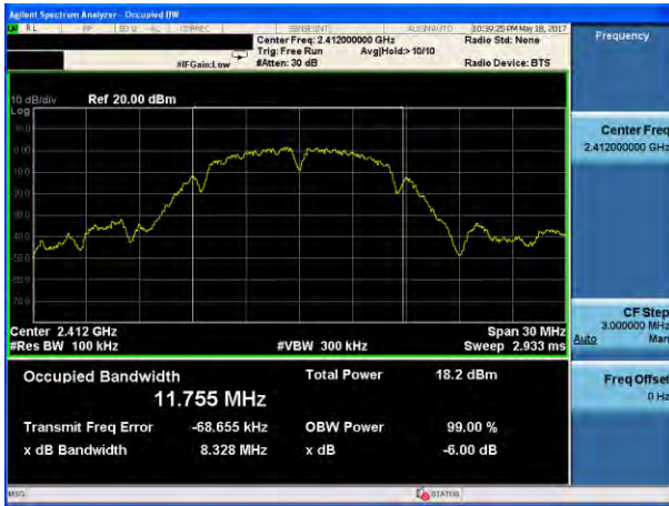
(802.11b) 6dB Bandwidth plot on channel 1
