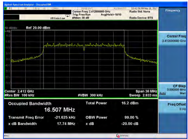
(802.11g) -20dB Bandwidth plot on channel 6
