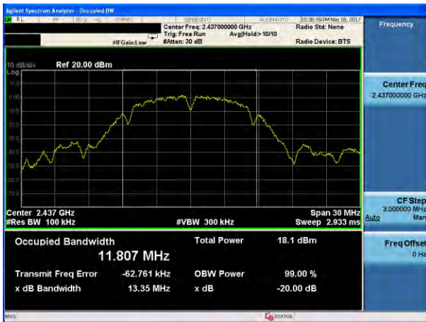
(802.11b) -20dB Bandwidth plot on channel 6
