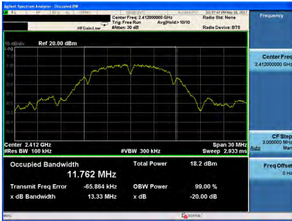
(802.11b) -20dB Bandwidth plot on channel 6
