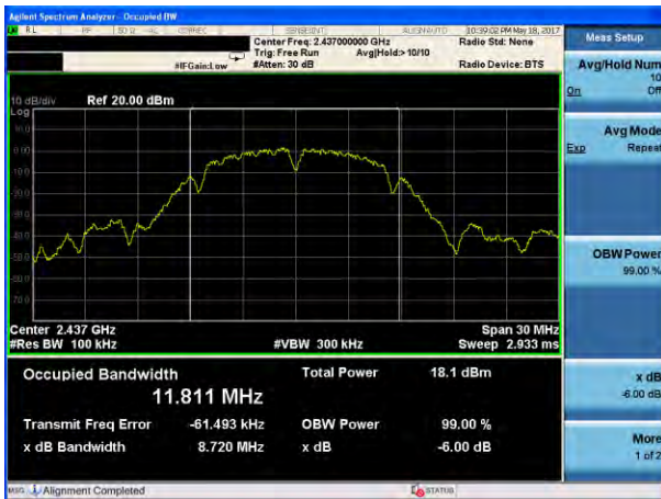
(802.11b) 6dB Bandwidth plot on channel 6
