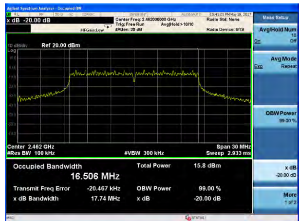
(802.11g) -20dB Bandwidth plot on channel 11
