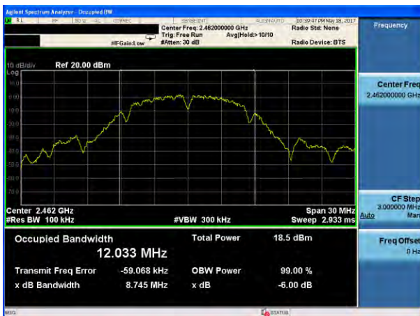
(802.11b) 6dB Bandwidth plot on channel 11
