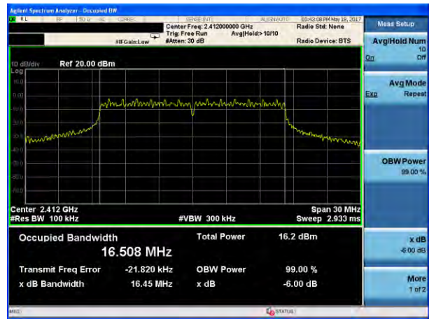
(802.11g) 6dB Bandwidth plot on channel 1
