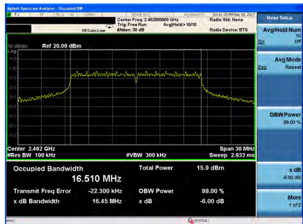
(802.11g) 6dB Bandwidth plot on channel 11
