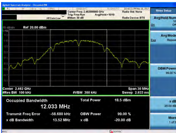
(802.11b) -20dB Bandwidth plot on channel 11
