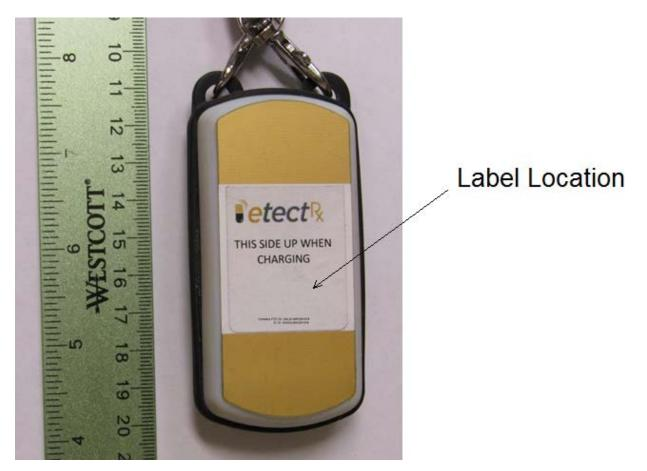
The module itself will not be labeled as it is too small. Therefore, the label will only be placed on the housing.
