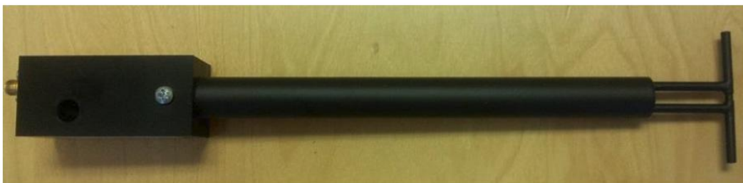
Figure 1 – MVG COMOSAR Validation Dipole
