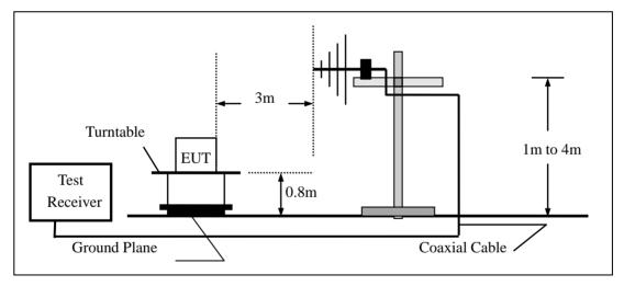
(c) For radiated emissions above 1000MHz
