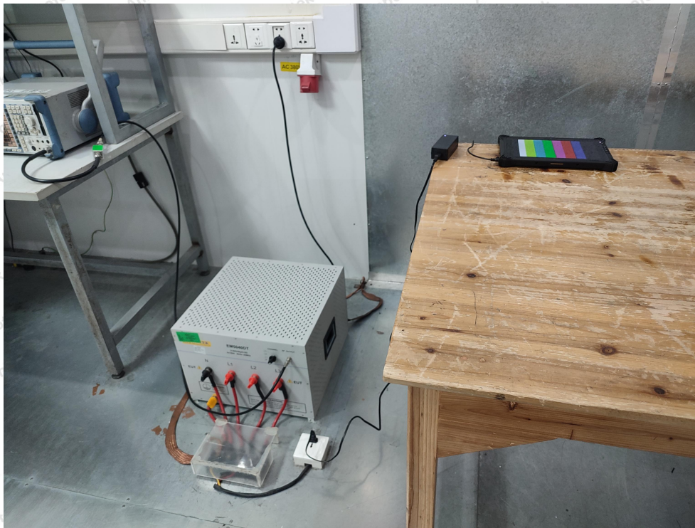
Photo of Conducted Emission Measurement
