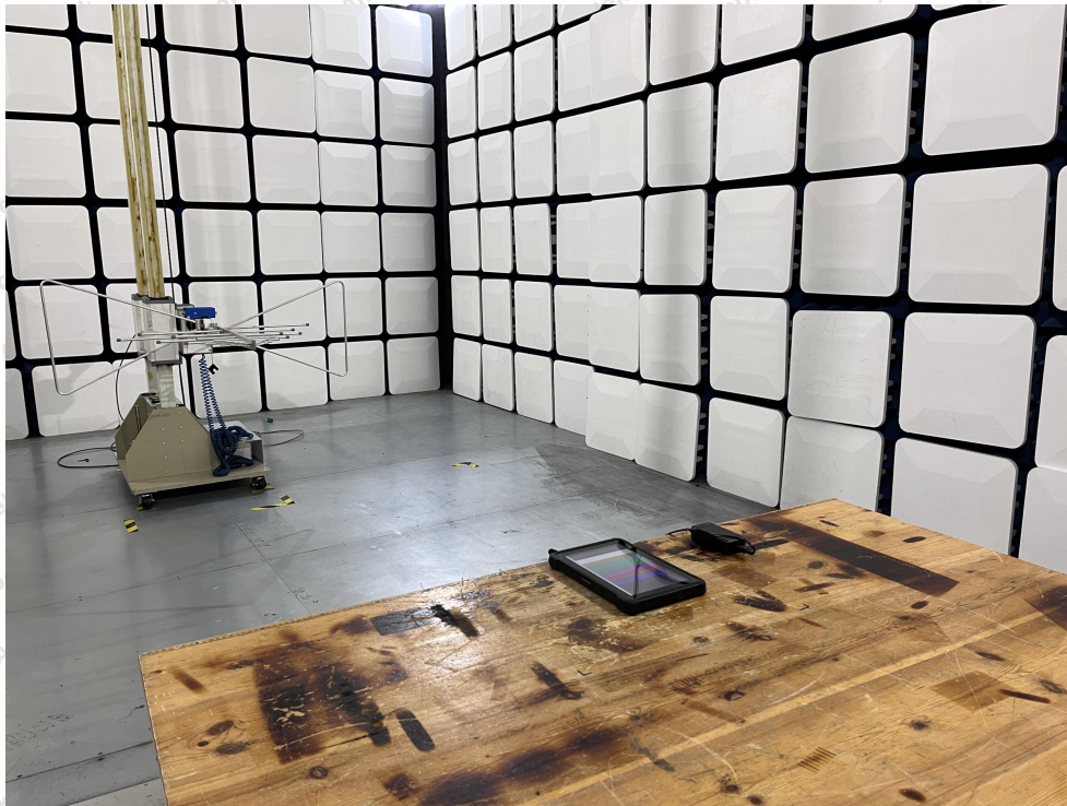
Photo of Radiation Emission Test
