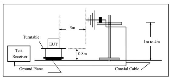
(c) For radiated emissions above 1000MHz
