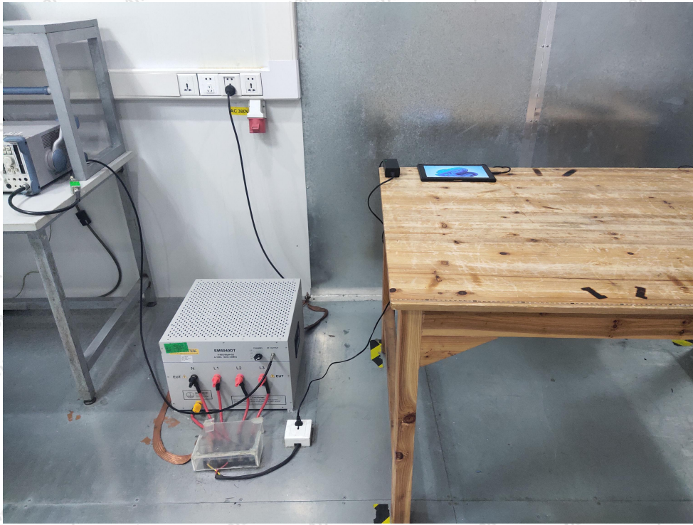
Photo of Conducted Emission Measurement
