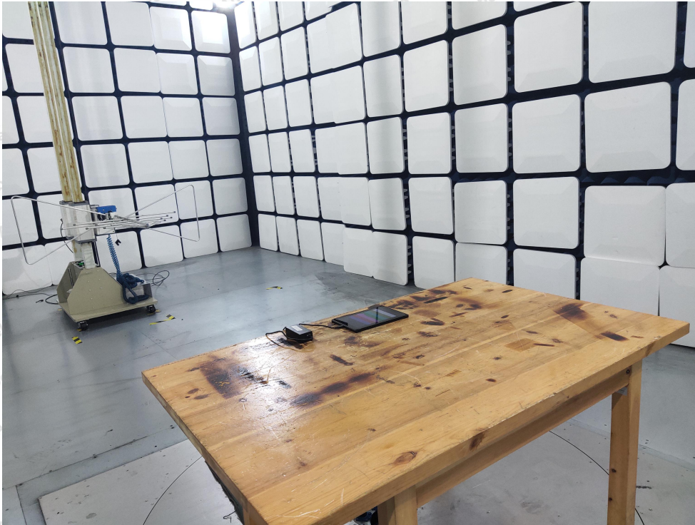
Photo of Radiation Emission Test
