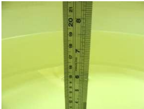
Photo of Liquid Height for Head SAR
