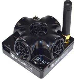
mobile beacons in the system, each beacon's location will be updated with the rate of  $16Hz/2 \sim 8Hz$ . If there are 3 mobile beacons =>  $16Hz/3 \sim 5Hz$ , etc. Future SW implementation will contain different solution that will improve update rate in the setup with multiple mobile beacons.
