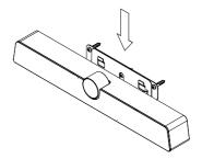
3) Use with panel: Fix the bracket onto the supporting bracket with screws, then place the integrated video conference terminal onto the bracket.(The bracket needs to be purchased separately.)
