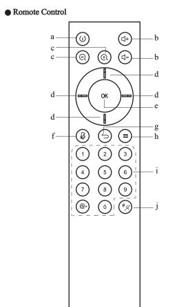
d. Direction Button: Press the direction buttons to move the camera or selection.
