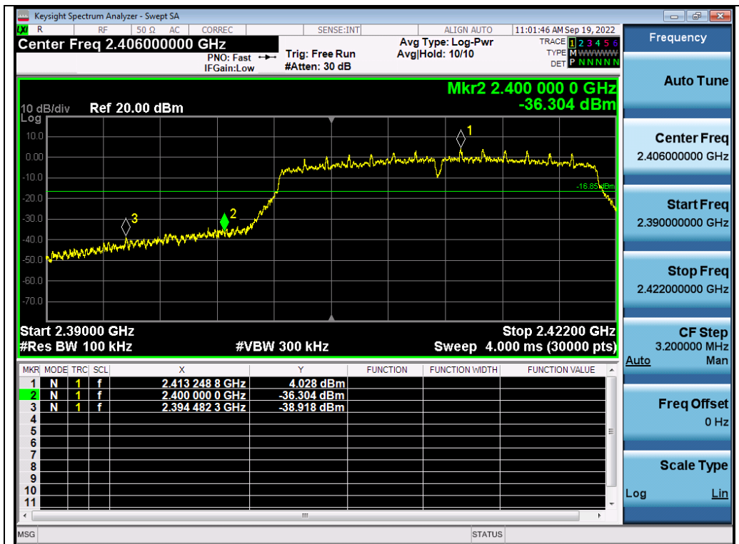
Test_Graph_802.11n20_ANT1_2412_MCS0_Lower Band Edge Emissions
