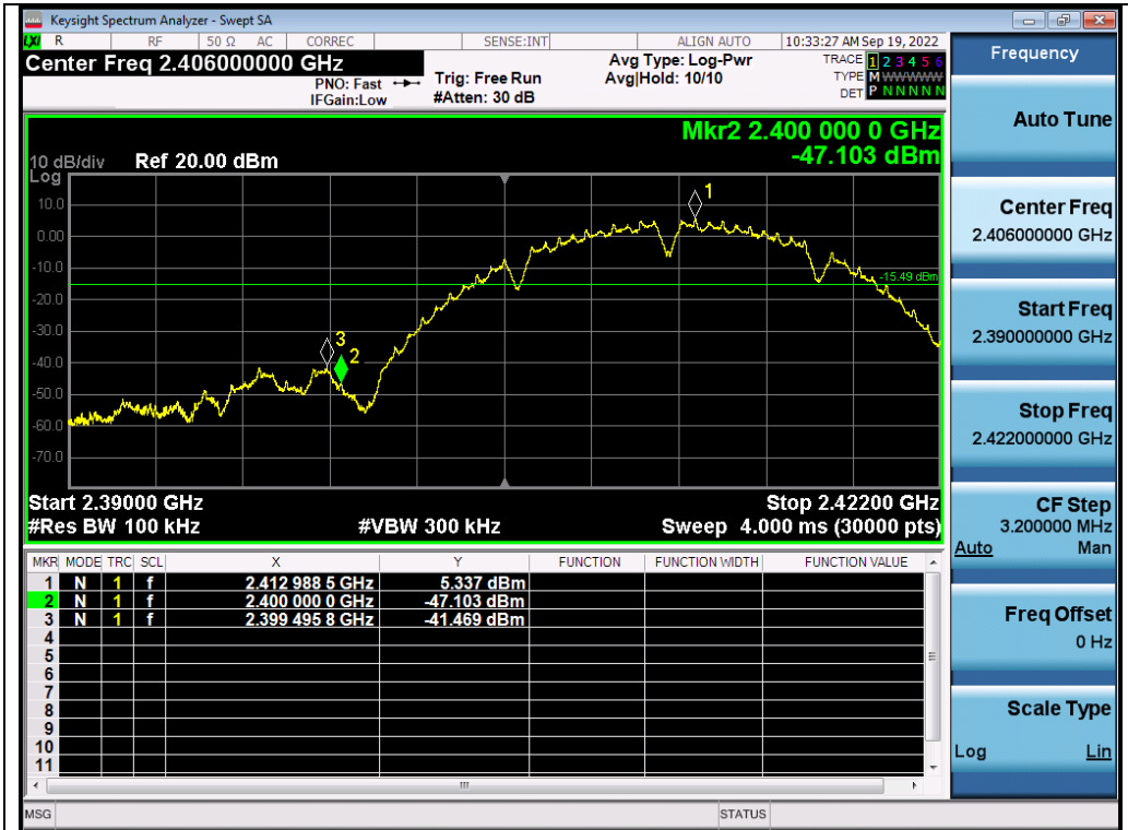
Test_Graph_802.11b_ANT1_2412_1Mbps_Lower Band Edge Emissions
