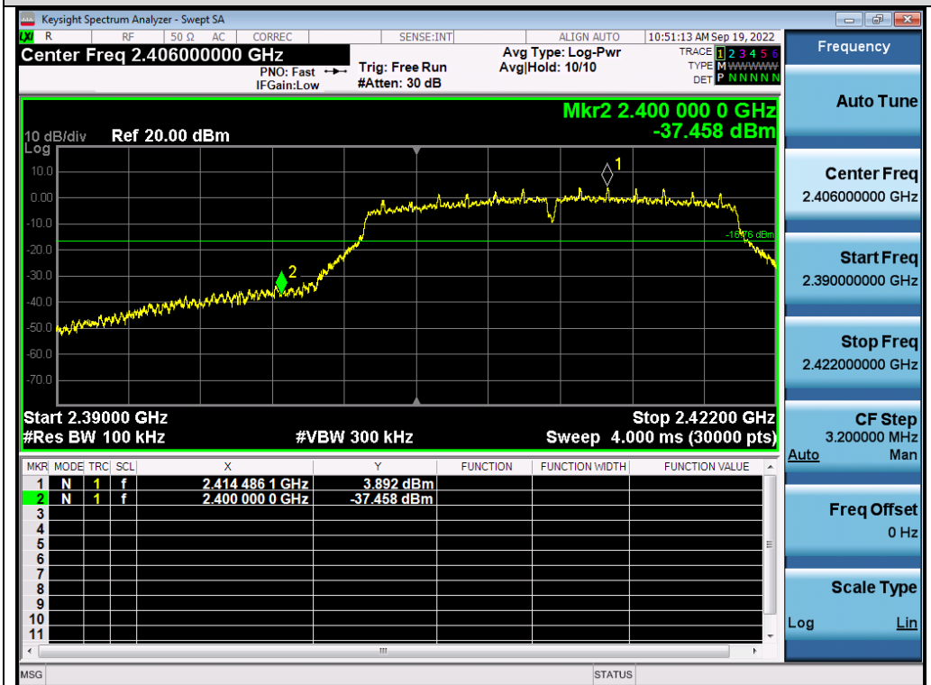
Test_Graph_802.11g_ANT1_2412_6Mbps_Lower Band Edge Emissions
