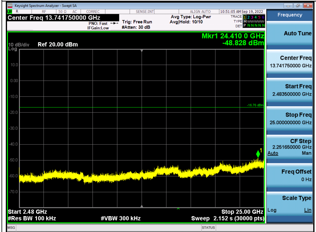
Test_Graph_802.11g_ANT1_2412_6Mbps_Higher Band Emissions
