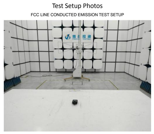
FCC RADIATED EMISSION TEST SETUP BELOW 1GHZ
