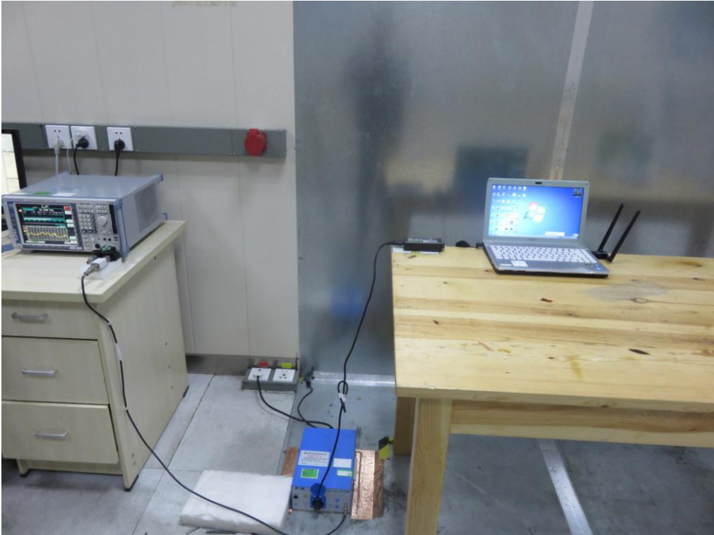
FCC RADIATED EMISSION TEST SETUP BELOW 1GHZ
