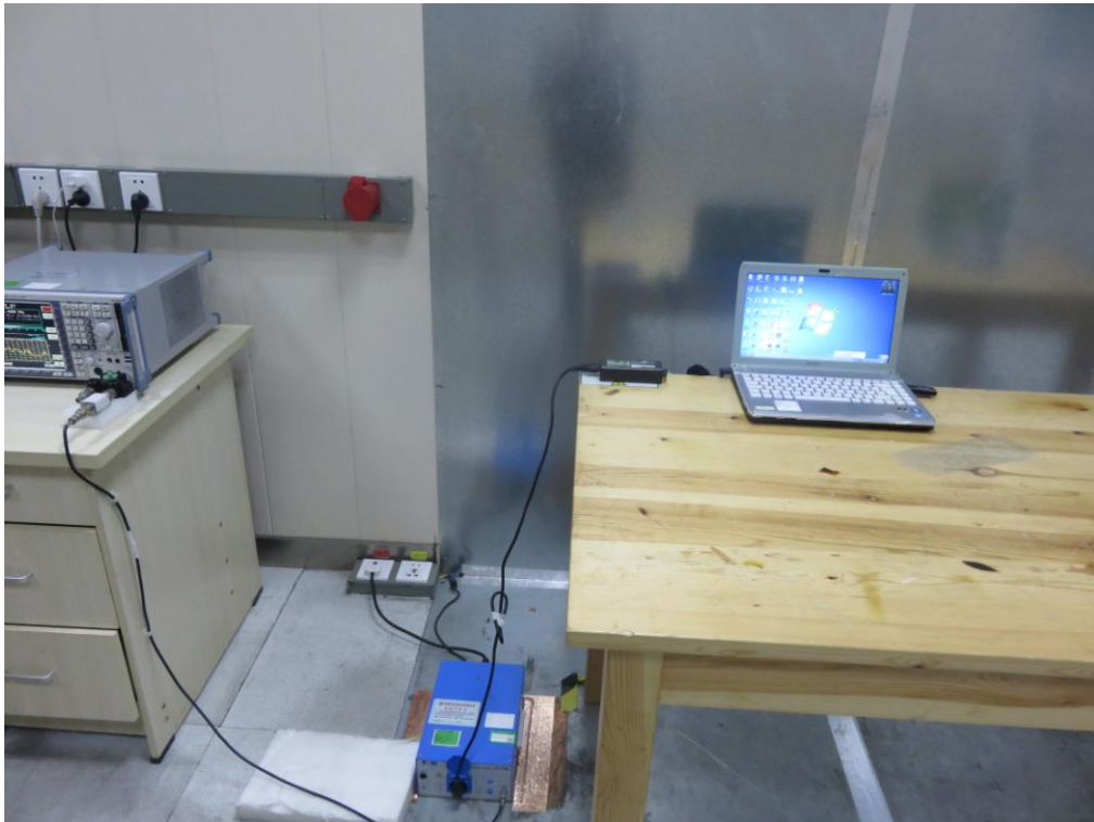
FCC RADIATED EMISSION TEST SETUP BELOW 1GHZ
