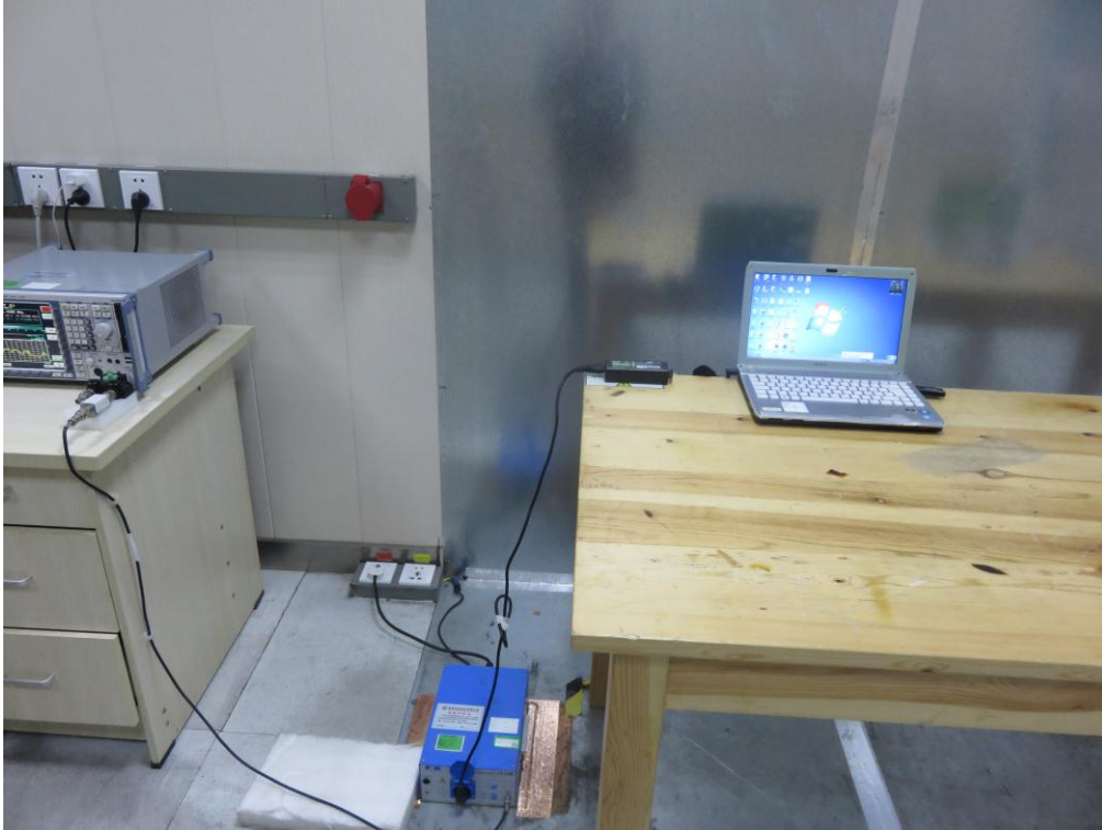
FCC RADIATED EMISSION TEST SETUP BELOW 1GHZ
