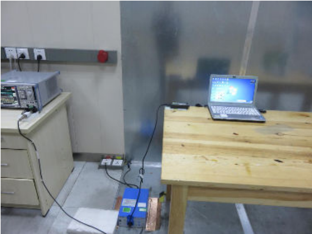
FCC RADIATED EMISSION TEST SETUP BELOW 1GHZ
