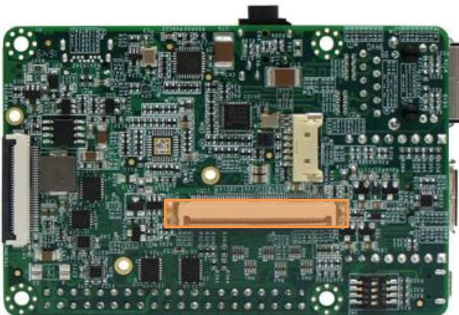
Figure 22 - PICO-PI-IMX7 LCD Display FPC Connector Location
