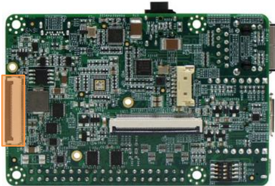
Figure 24 - PICO-PI-IMX7 Touch Panel Connector Location
