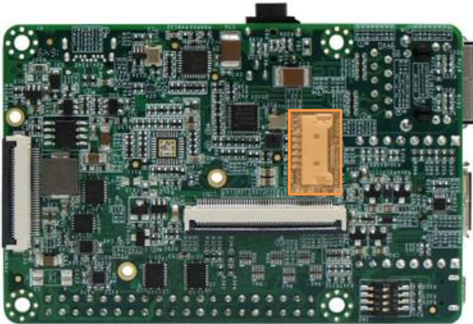
Figure 23 - PICO-PI-IMX7 Touch Panel Connector Location
